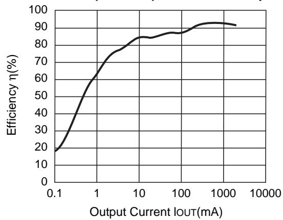
**R1224N332L ( $V_{IN}=4.8V$ ) CDRH127-27 $\mu$ H**
