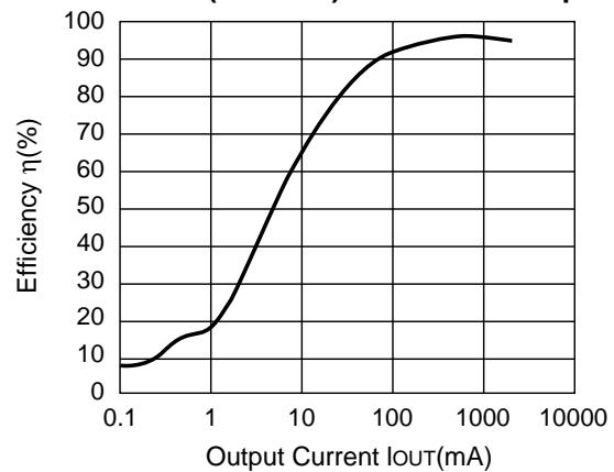
R1224N502M ( $V_{IN}=12V$ ) CDRH127-27 $\mu$ H
