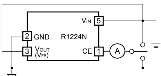
**Output Delay Time for Protection Circuit**
