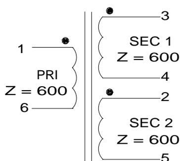
BOTH SECONDARIES MUST BE LOADED FOR IMPEDANCE SPECIFICATIONS TO BE ACCURATE.
