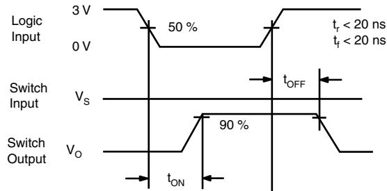
Figure 1. Single Supply Switching Time
