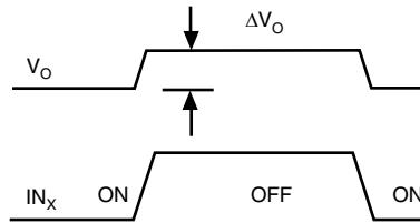
$\Delta V_O$  = measured voltage error due to charge injection
