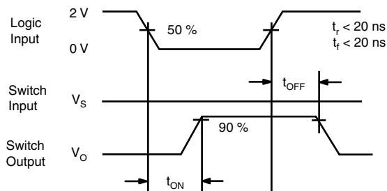
**Figure 2. Dual Supply Switching Time**
