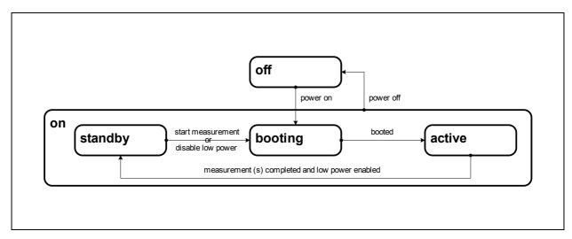
In continuous run mode (see Register SENS\_RUN) or when low power is disabled (see Register SYS\_CTRL), the device remains in *active* state.
