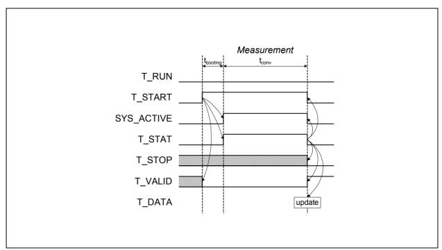
Signal T\_RUN is written low to select a single shot measurement. Note that T\_STOP is typically low (cleared by a previous measurement), but its state is ignored in a single shot measurement. T\_START is written high to start measuring: T\_VALID in T\_VAL is cleared and the device starts *booting* to *active*. Once active SYS\_ACTIVE goes high, and measurement starts (T\_STAT goes high).
