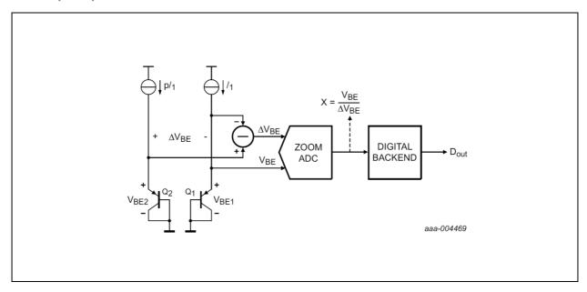
The temperature is measured using a high-precision (12 bits) zoom-ADC. The analog part is able to measure a strongly temperature dependent  $X = V_{BE}/\Delta V_{BE}$ . The X is found by first applying a coarse search (successive approximation), and then a sigma-delta in a limited range. The accuracy of the sensor is shown in Figure 12. The conversion time is shown in Figure 9.
