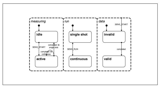
When in the *single shot* run mode, starting a measurement is under control of the master. By default a sensor is idle; it can be started by writing a 1 to the corresponding bit in SENS\_START. After a start, the sensor stops when the measurement is completed. Whether a sensor is idle or active measuring can be detected by reading SENS\_STAT. The measured values can be obtained via their respective readout registers (T\_VAL and H\_VAL). Writing to SENS\_STOP in single shot has no effect.
