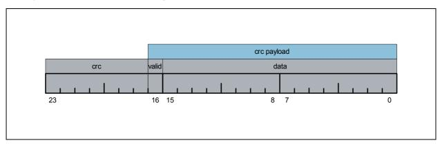
The *checksum* is a cyclic redundancy check over the data and the valid flag; the stored checksum is the result of CRC-7 (polynomial x7+x3+1, see https://en.wikipedia.org/wiki/Cyclic\_redundancy\_check) with 0x7F as initial vector (i.e. with all bits flipped), see Computing CRC-7 for sample C code.
