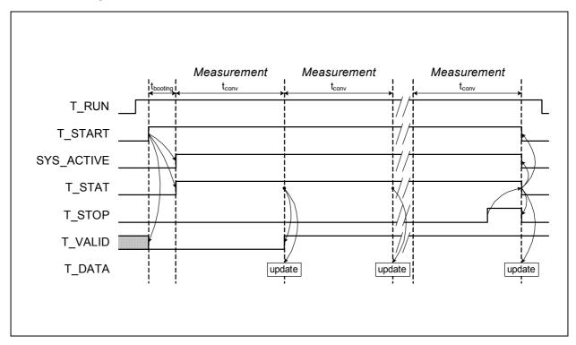
Figure 19 shows the timing of a continuous T measurement.
