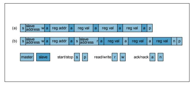
A typical write transaction (see Figure 16 a) therefore has the following format. The master initiates a transaction with a so-called start condition "s". This blocks the bus. Next, the master sends the 7 bits ENS210 slave address followed by a 1 bit direction (a 0 indicating write "w"). This byte is acknowledged "a" by the slave. The master continues by sending the 8 bit register address, which is acknowledged by the slave.
