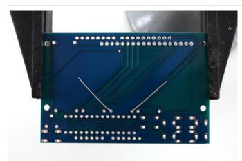
Bend the 'legs' of the resistor out so it sits flat against the PCB and flip it over.
