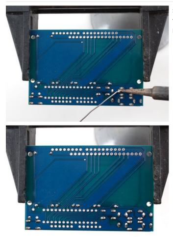
Solder each leg, taking care not to accidentally 'short' two button legs together. The ones for the directional pads are very close!
