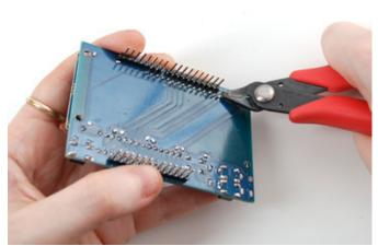
Finish up by carefully clipping the leads. For some Arduinos, the long leads may interfere with headers or parts on the Arduino board so we suggest just clipping them all. Do it carefully as these are a little difficult to cut and may fly at you. We suggest doing it over a trash can.
