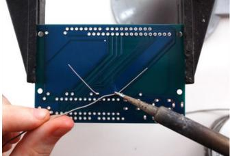
With your soldering iron heated up and ready, solder in both leads of the resistor. To do this, heat up the round ring pad and the wire lead at the same time for 2 or 3 seconds, then dip the end of the solder into the heated joint to melt it in.
