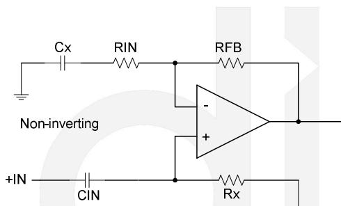
**Figure 3 Non-Inverting Gain Configuration**
