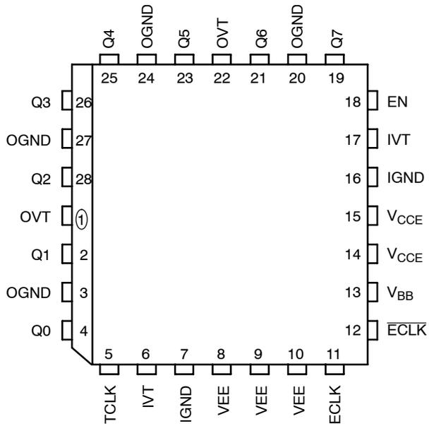
**Figure 1. Pinout: PLCC-28**
