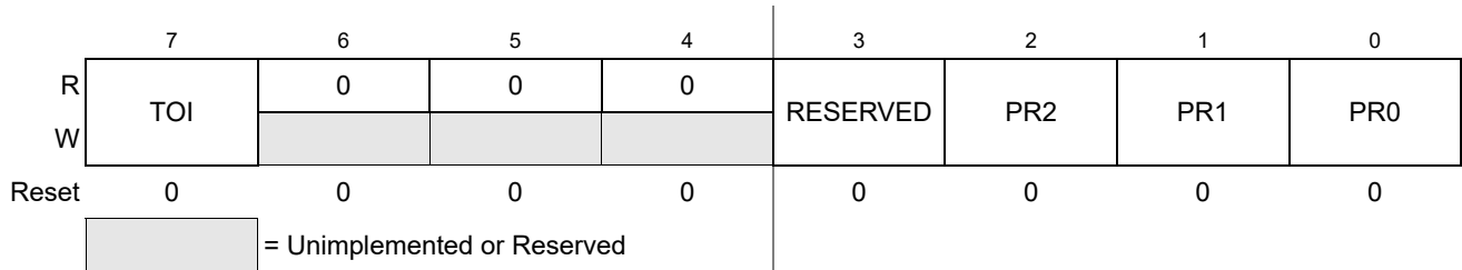
Figure 11-15. Timer System Control Register 2 (TSCR2)
