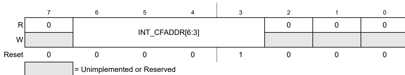
Figure 4-4. Interrupt Configuration Address Register (INT_CFADDR)
