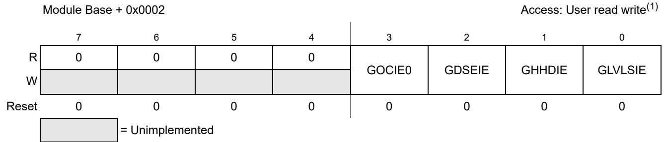
Figure 17-5. GDU1PHV1 Interrupt Enable Register (GDUIE)
