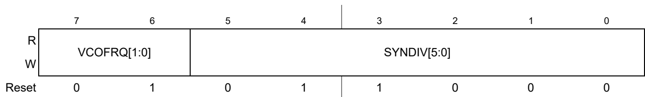
Figure 8-7. S12CPMU_UHV_V11 Synthesizer Register (CPMUSYNR)
