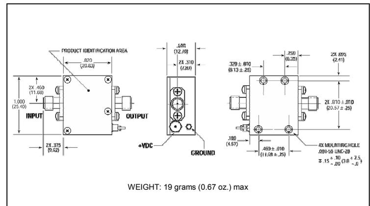
\* Dimensions are inches (millimeters) ±0.015 (0.38) unless otherwise specified.
