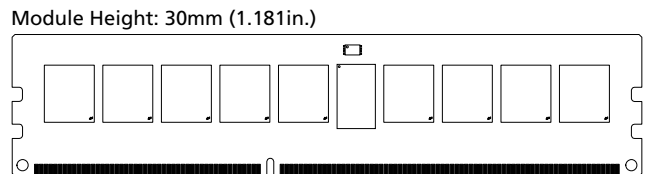
Figure 2: 240-Pin RDIMM (MO-269 R/C B1)
