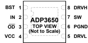
Figure 5. 8-Lead LFCSP Pin Configuration
