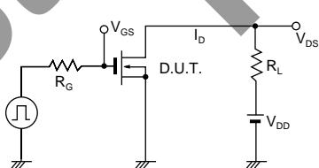
Fig.13 Switching Time Test Circuit
