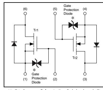
(1) Tr1 Source (2) Tr1 Gate (3) Tr2 Drain (4) Tr2 Source
