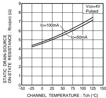
Fig.7 Static Drain-Source On-State Resistance vs. Channel Temperature
