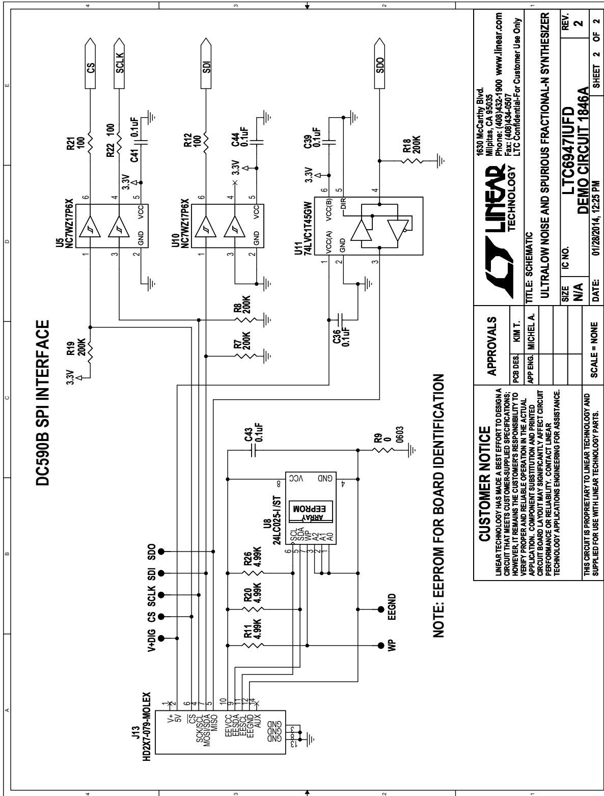
**Note:** The buffers shown on sheet 2 of 2 of the schematic are used to protect the LTC6947 when connected to the DC590 before the LTC6947 is powered up. There is no need for such circuitry if the SPI bus is not powered before powering up the LTC6947. The EEPROM is for identification and is not needed to program the LTC6947.
