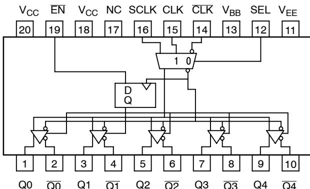
Warning: All V<sub>CC</sub> and V<sub>EE</sub> pins must be externally connected to Power Supply to guarantee proper operation.
