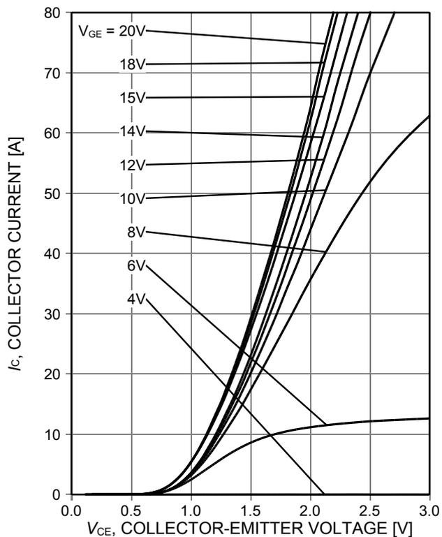
Figure 3. Typical output characteristic ( $T_{vj} = 25^\circ\text{C}$ )
