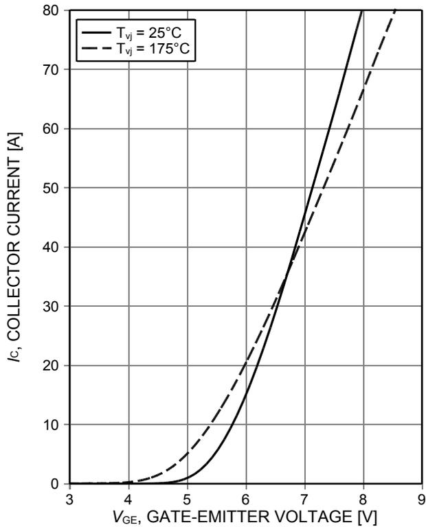
Figure 5. **Typical transfer characteristic**
