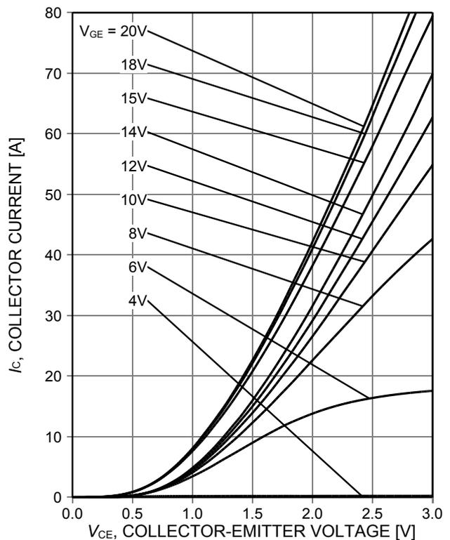
Figure 4. Typical output characteristic ( $T_{vj} = 150^\circ\text{C}$ )
