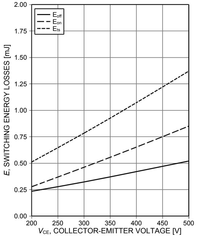
Figure 14. **Typical switching energy losses as a function of collector emitter voltage** (inductive load,  $T_{vj}=150^\circ C$ ,  $V_{GE}=15/0V$ ,  $I_C=28A$ ,  $r_G=34\Omega$ , Dynamic test circuit in Figure E)
