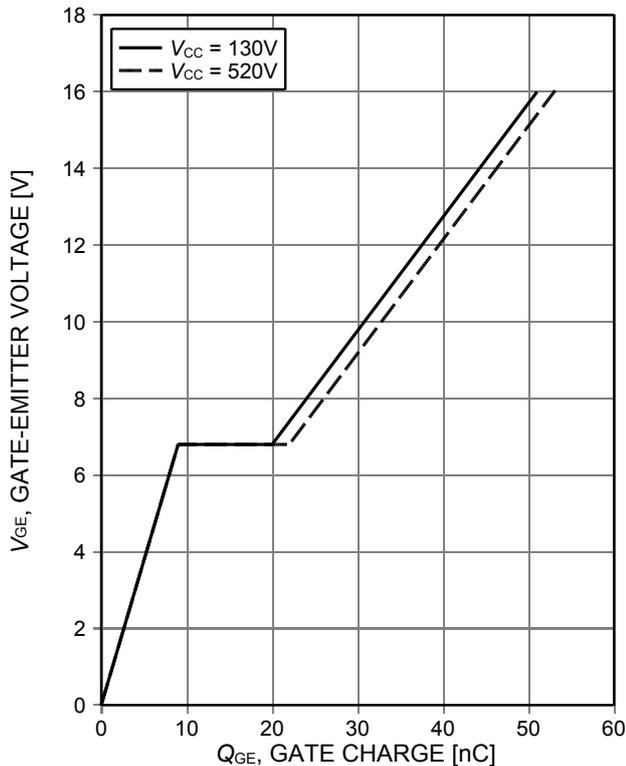
Figure 15. **Typical gate charge** ( $I_C=28A$ )
