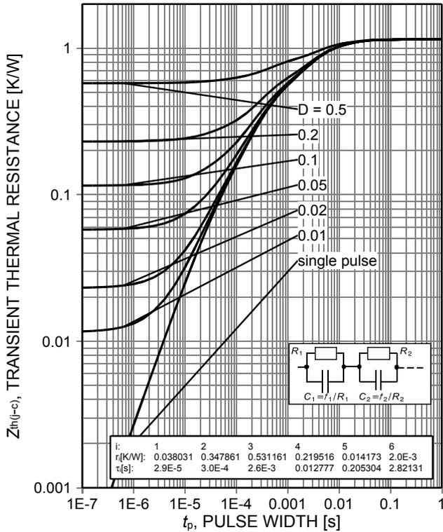
Figure 17. IGBT transient thermal resistance ( $D=t_p/T$ )
