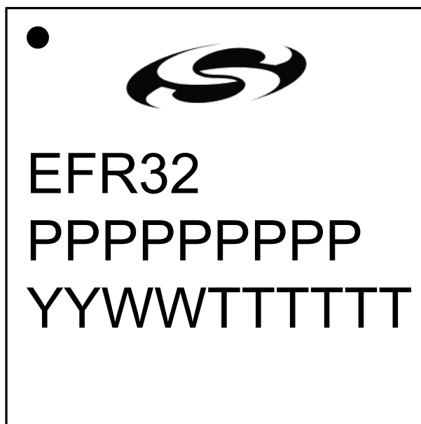
Figure 8.3. QFN32 Package Marking
