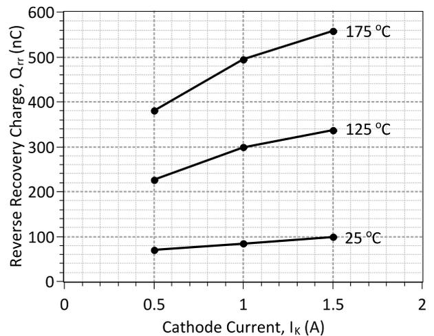
**Figure 6: Reverse Recovery Charge vs Cathode Current**
