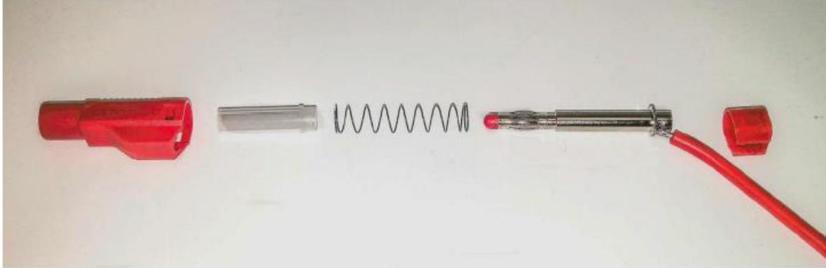
Note: Use very short wire strip length and solder just above the spring retainer.
