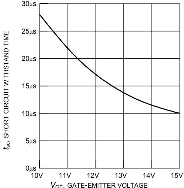
**Figure 19. Short circuit withstand time as a function of gate-emitter voltage**
