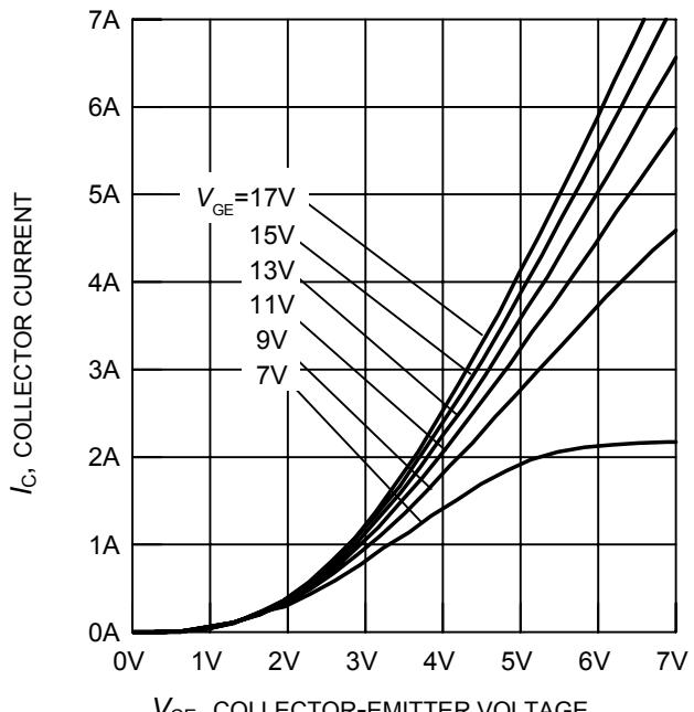
**Figure 6. Typical output characteristics**
