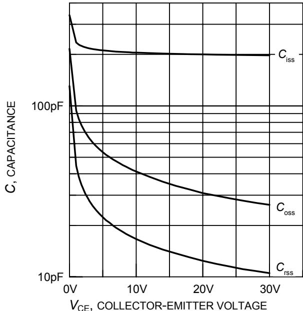
**Figure 18. Typical capacitance as a function of collector-emitter voltage**
