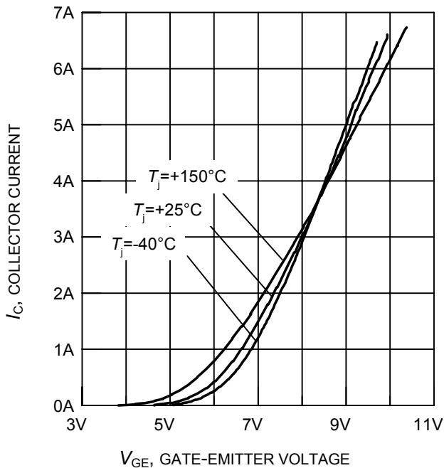
**Figure 7. Typical transfer characteristics**
