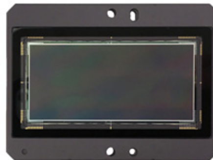
Figure 1. KAI-50140 CCD Image Sensor
