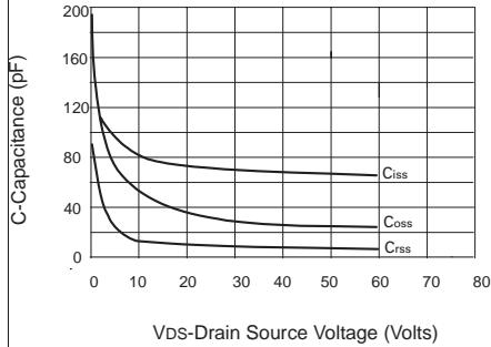
**Capacitance v drain-source voltage**
