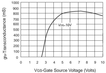
**Transconductance v gate-source voltage**
