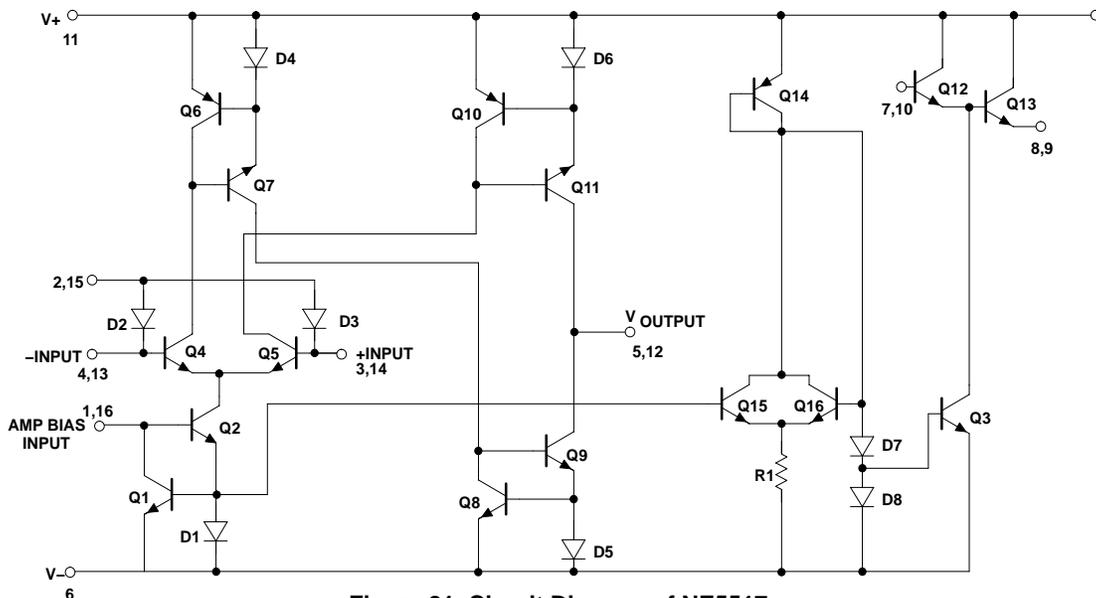
Figure 21. Circuit Diagram of NE5517
