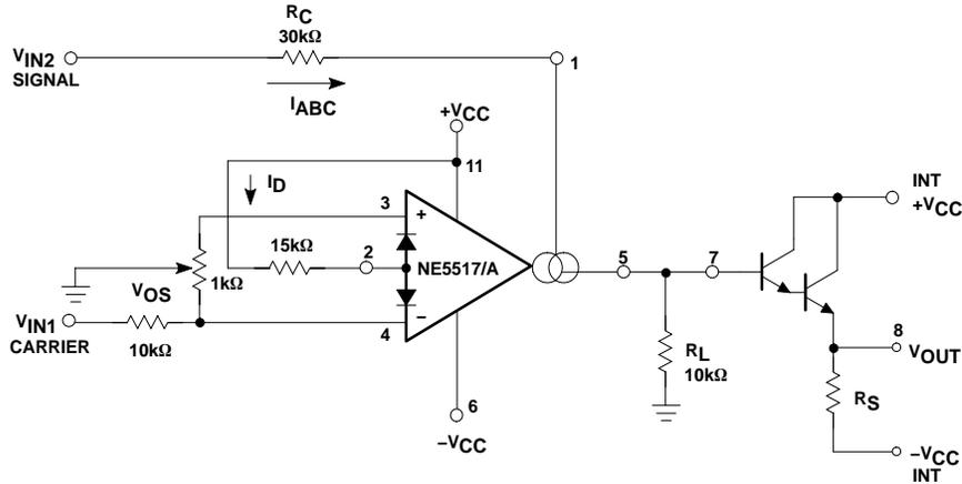
Figure 25. Amplitude Modulator
