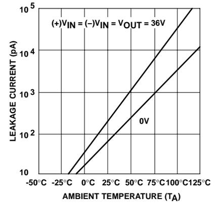
Figure 8. Leakage Current
