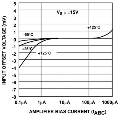
Figure 3. Input Offset Voltage
