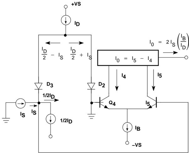
Figure 22. Linearizing Diode
