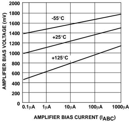
Figure 12. Amplifier Bias Voltage vs. Amplifier Bias Current
