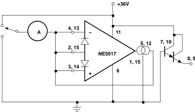
Figure 17. Leakage Current Test Circuit
