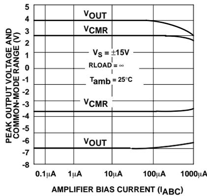
Figure 7. Peak Output Voltage and Common-Mode Range
