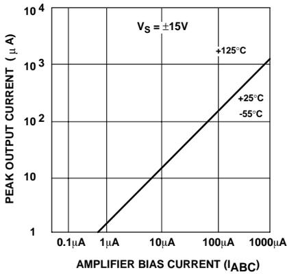
Figure 6. Peak Output Current
