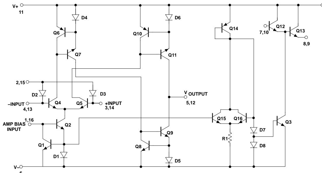
Figure 21. Circuit Diagram of NE5517
