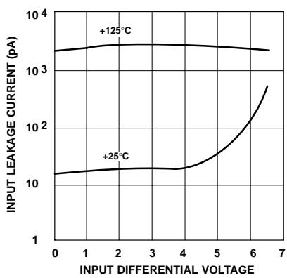
Figure 9. Input Leakage
