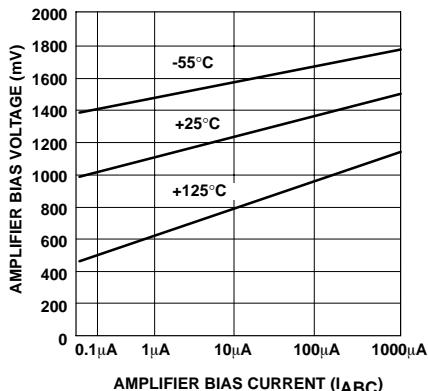
Figure 12. Amplifier Bias Voltage vs.
