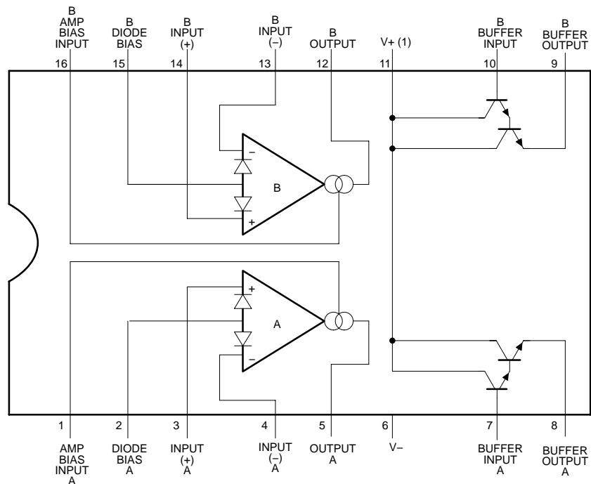
NOTE: V+ of output buffers and amplifiers are internally connected.
