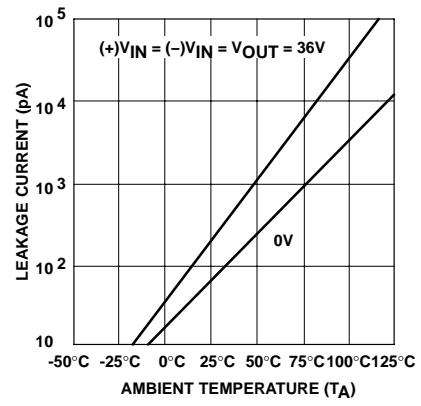
Figure 8. Leakage Current
