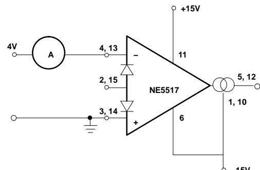
Figure 18. Differential Input Current Test Circuit
