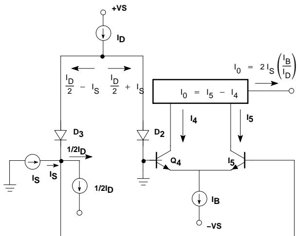
Figure 22. Linearizing Diode
