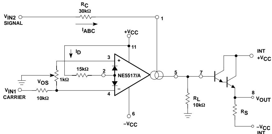
**Figure 25. Amplitude Modulator**
