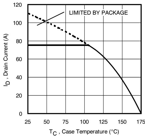
**Fig 9.** Maximum Drain Current vs.
