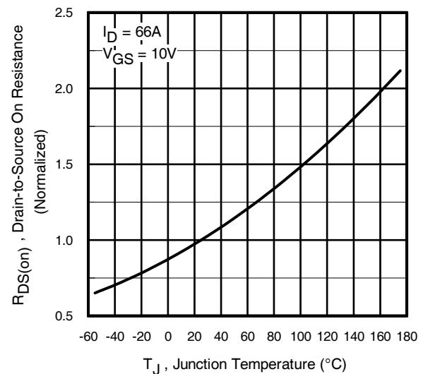
**Fig 10.** Normalized On-Resistance
