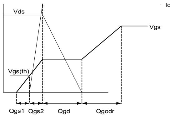
**Fig 13b.** Gate Charge Waveform
