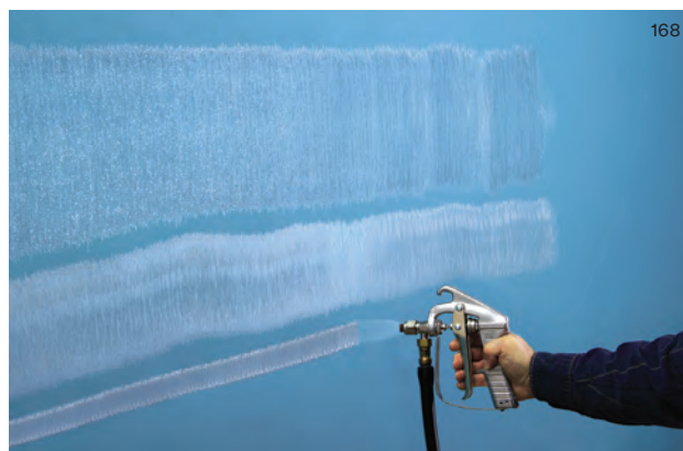
Spray patterns from 1–18+\" are achievable using 3M™ Cylinder Spray Adhesives and various spray tips.
