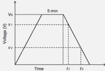
$$C = \frac{I \times (t_2 - t_1)}{v_1 - v_2}$$
