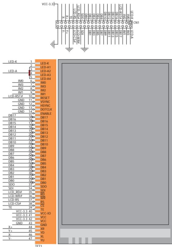
Figure 2: TFT PROTO schematic
