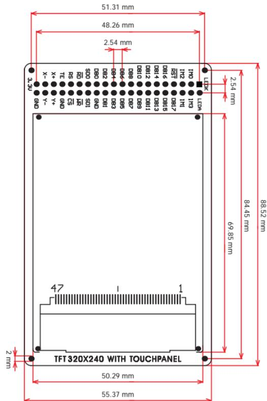
Figure 3: TFT PROTO dimensions
