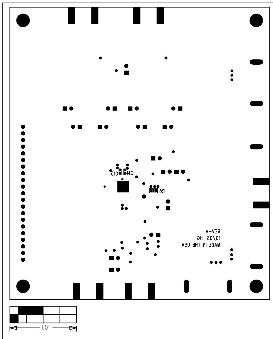
Figure 9. MAX5858A EV Kit Component Placement Guide—Solder Side
