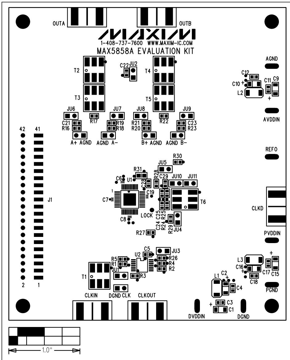
Figure 4. MAX5858A EV Kit Component Placement Guide—Component Side
