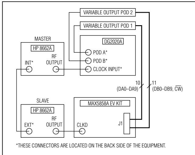
Figure 1. Quick Start Setup for PLL Disabled Mode
