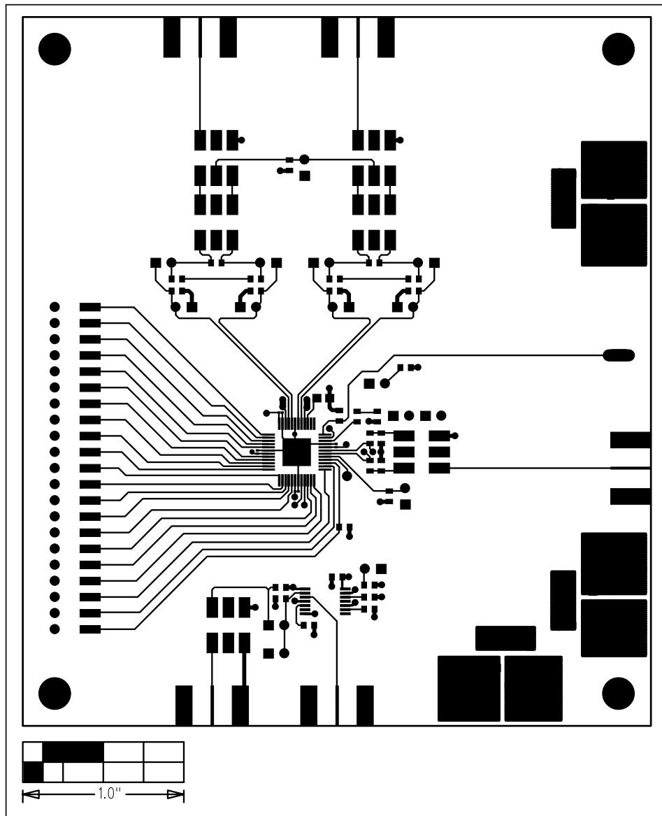
Figure 5. MAX5858A EV Kit PCB Layout—Component Side
