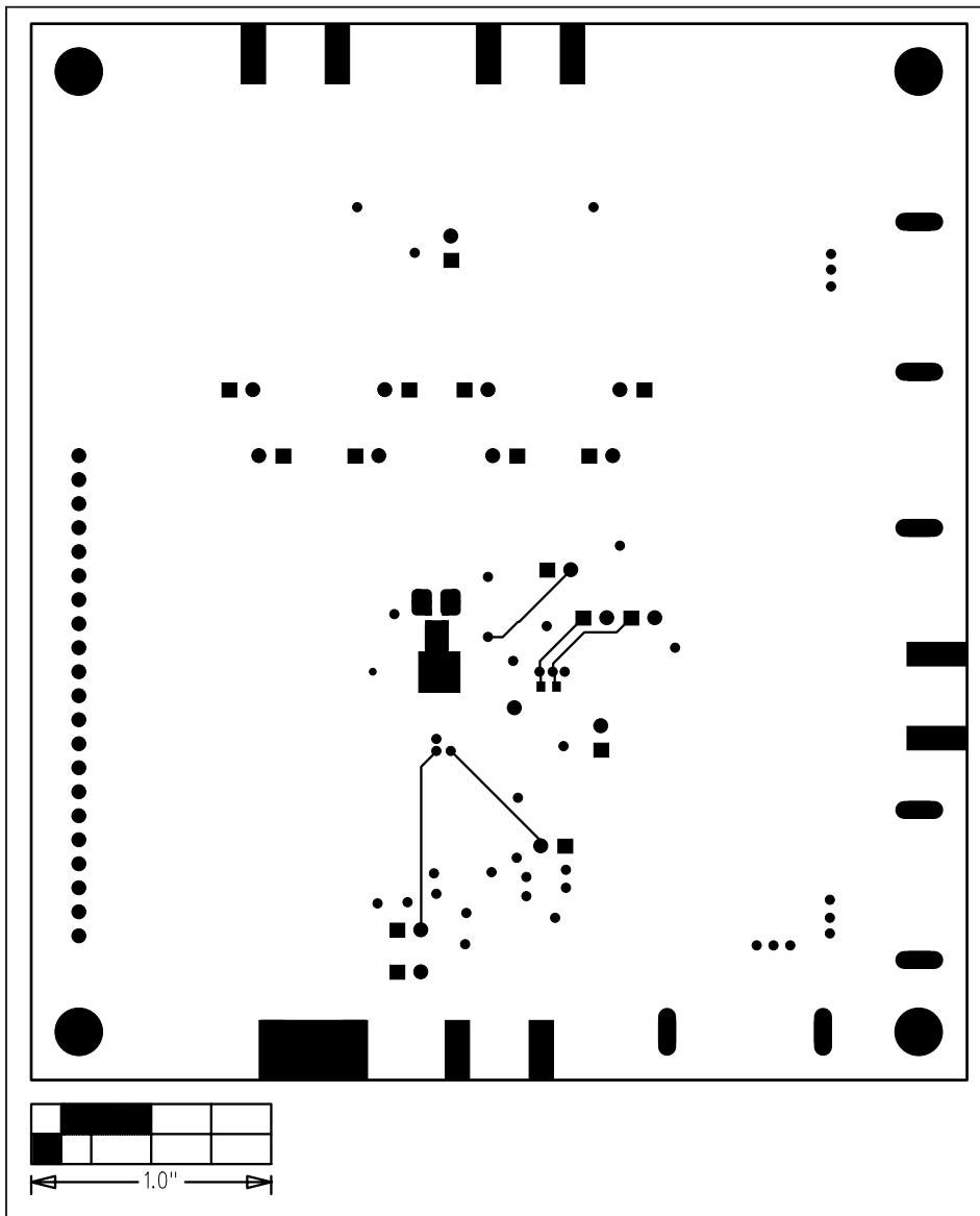
Figure 8. MAX5858A EV Kit PCB Layout—Solder Side
