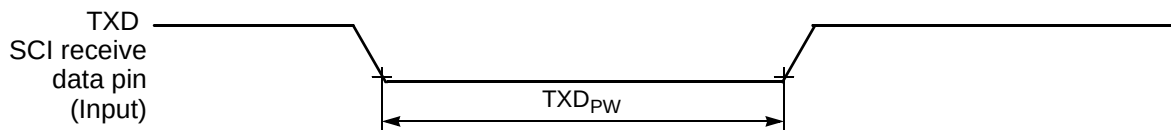
Figure 10-16 TXD Pulse Width
