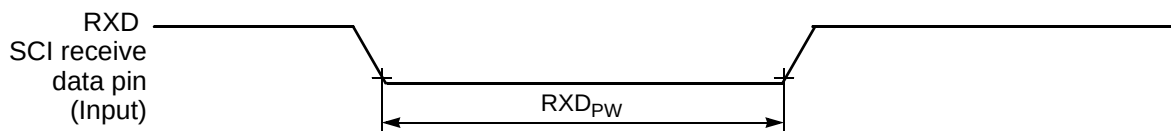
Figure 10-15 RXD Pulse Width
