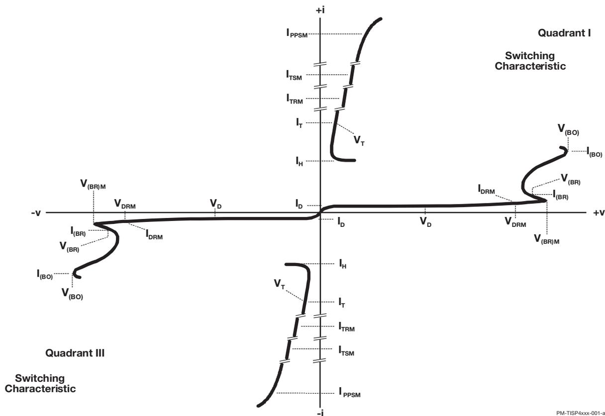
Figure 1. Voltage-Current Characteristic for T and R Terminals
