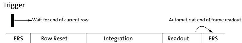
Figure 16: Entering and Leaving a Global Reset Sequence
