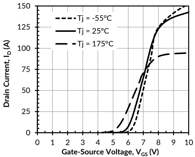
Figure 6. Typical transfer characteristics at  $V_{DS} = 5\text{V}$
