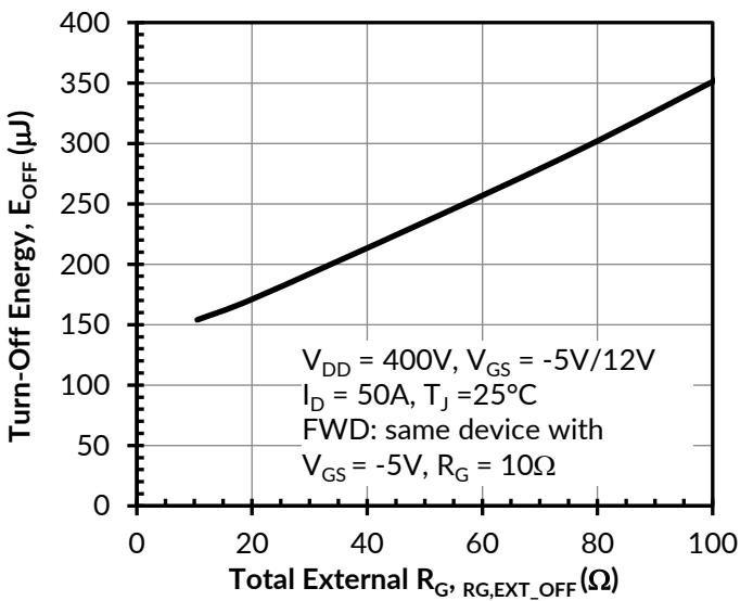
Figure 20. Clamped inductive switching turn-off energy vs.  $R_{G,EXT\_OFF}$
