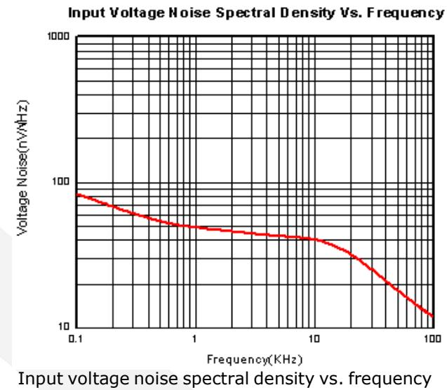
Input voltage noise spectral density vs. frequency
