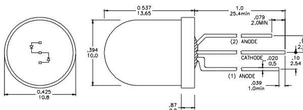
\* Tolerance :  $\pm \frac{0.01}{0.25}$  Unit :  $\pm \frac{\text{inch}}{\text{mm}}$
