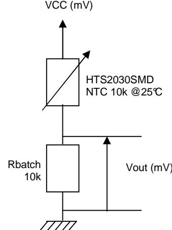
$$V_{OUT} (mV) = \frac{Vcc(mV) * R_{batch}(\Omega)}{R_{batch}(\Omega) + NTC_{HTS\ 2030SMD}(\Omega)}$$
