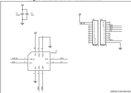
Figure 1. STEVAL- MKI142V1 circuit schematic
