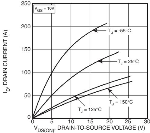
Figure 1, Output Characteristics
