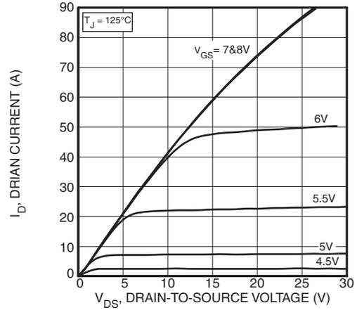
Figure 2, Output Characteristics
