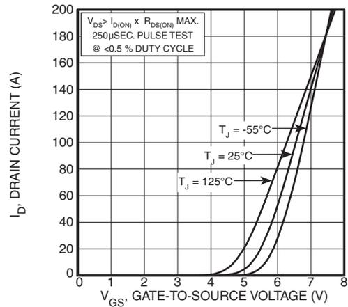
Figure 4, Transfer Characteristics
