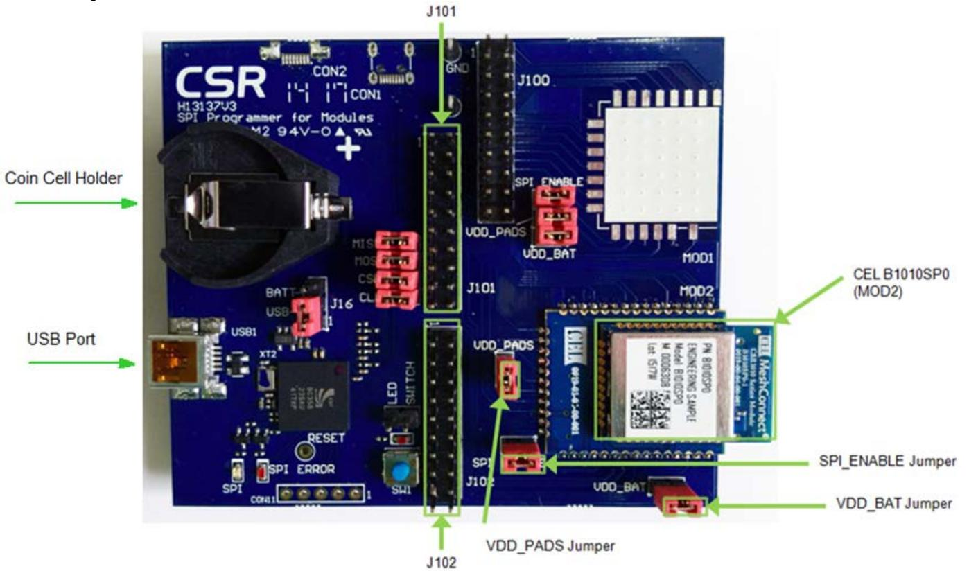
**Figure 1 - Evaluation Kit Target Board**
