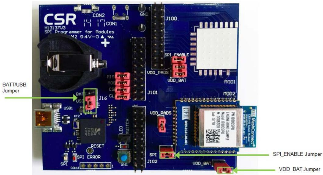
**Figure 26 - SPI\_ENABLE, VDD\_BAT, BATT/USB Jumper Settings**
