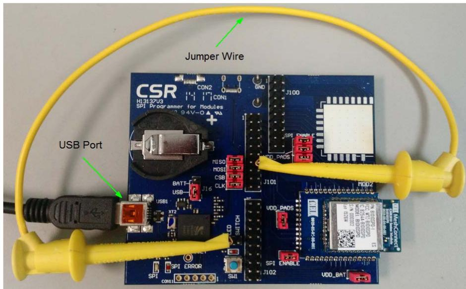
**Figure 20 - Evaluation Kit Target Board Showing USB Port Location & Jumper Wire**
