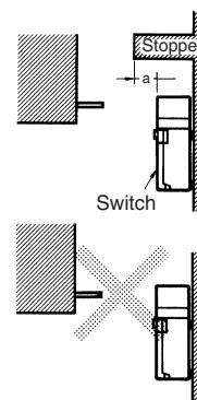
Refer to *Dimensions* for the mounting dimension of the Operation Key and mount the Operation Key correctly. The Operation Key will soon become damaged or worn out if it is not mounted correctly.
