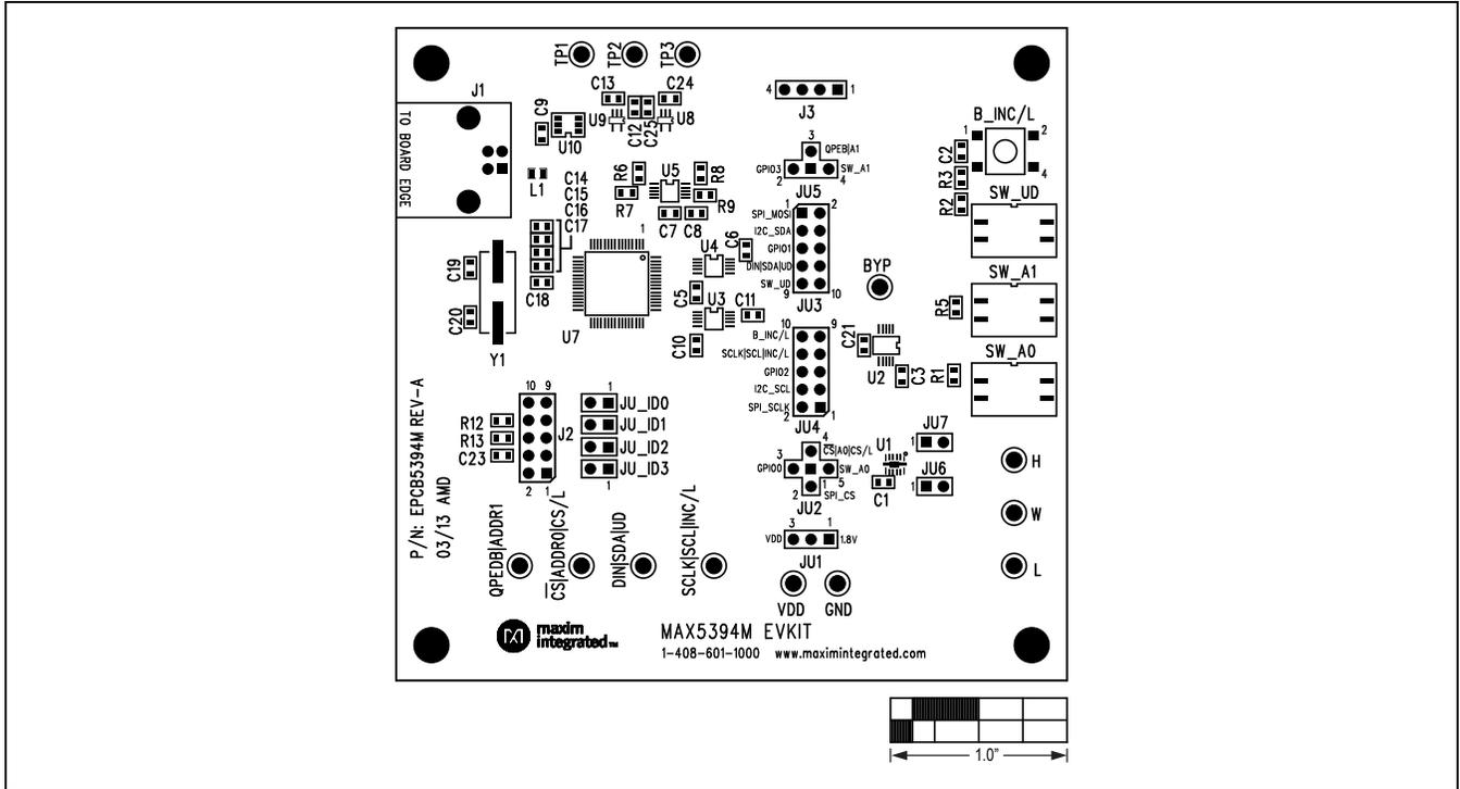
Figure 3. MAX5394M EV Kit Component Placement Guide—Component Side
