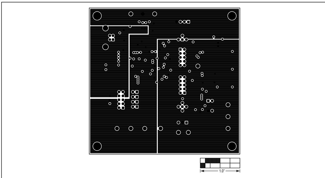
Figure 6. MAX5394M EV Kit PCB Layout—Inner Layer 3
