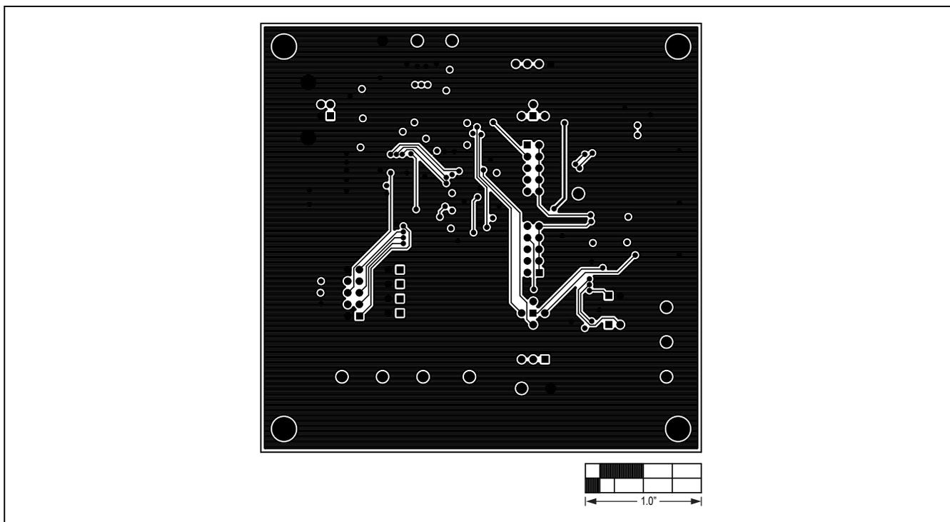
Figure 7. MAX5394M EV Kit PCB Layout—Solder Side
