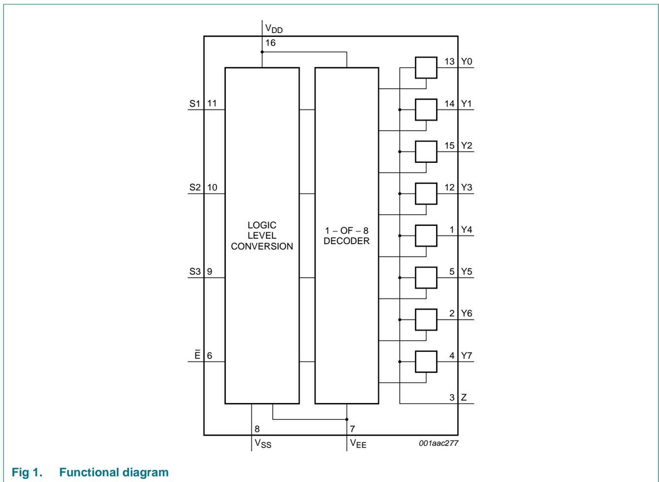
**Fig 1. Functional diagram**
