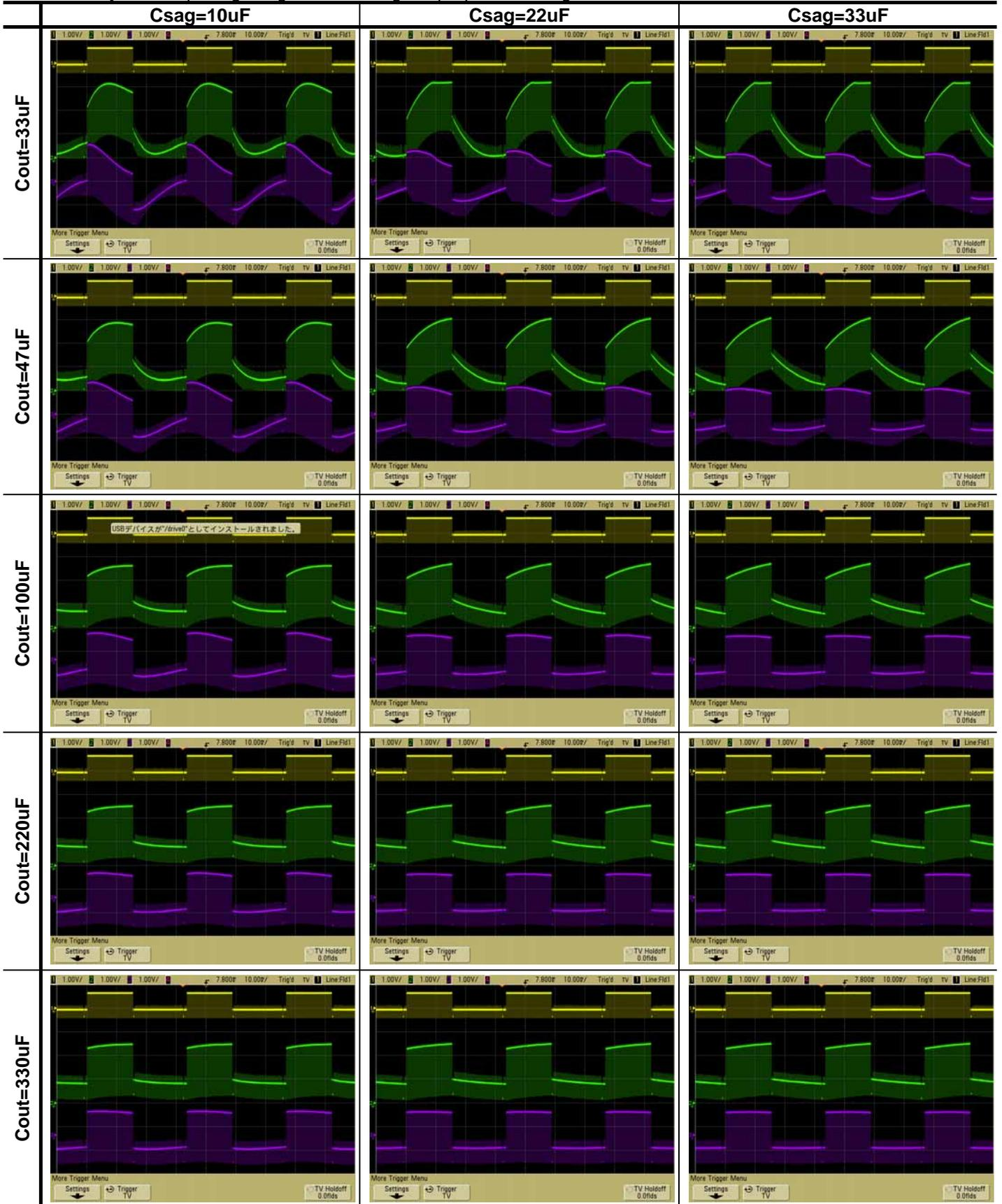
Input signal: bounce signal (IRE0%, IRE100%, 30Hz), resistance=150Ω
