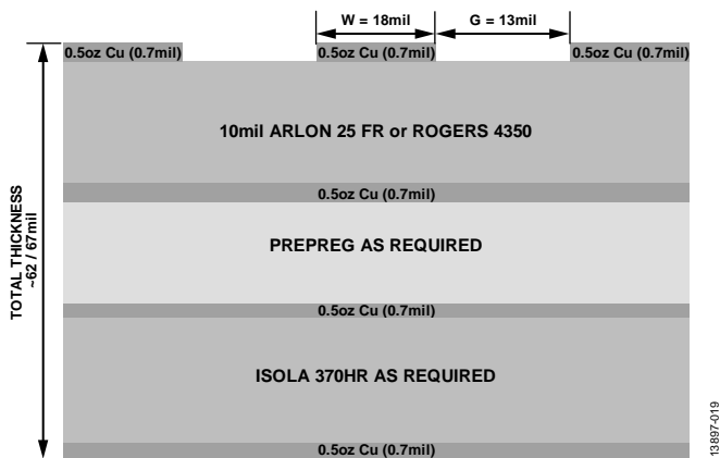
Figure 94. Evaluation Board Cross Sectional View
