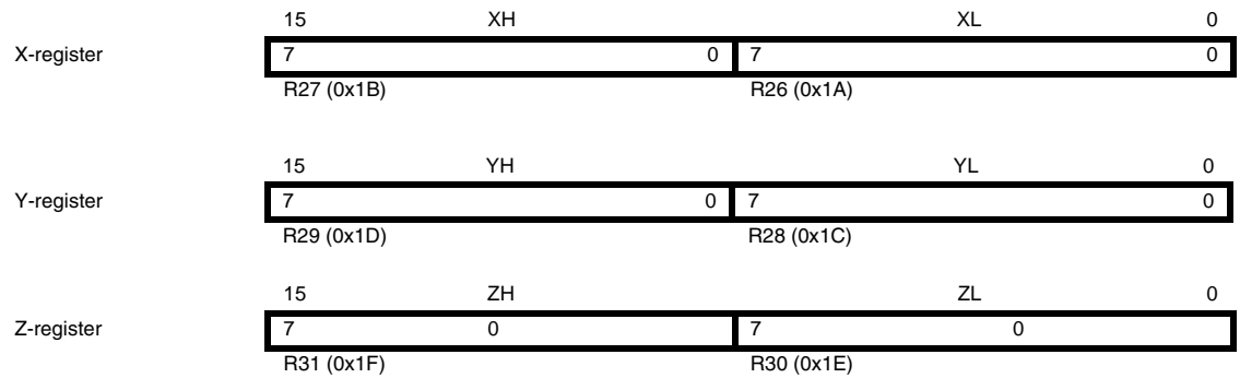
Figure 5-5. The X-, Y-, and Z-registers
