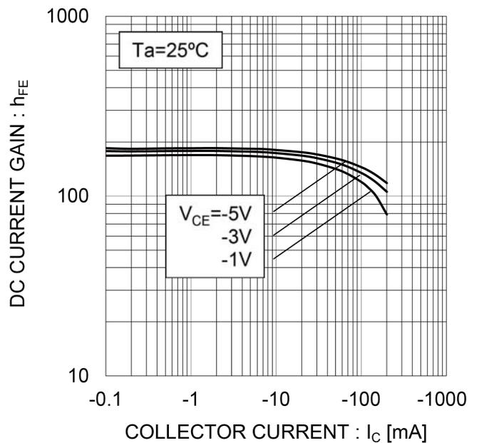
● **Electrical characteristic curves** ( $T_a=25^\circ\text{C}$ )
