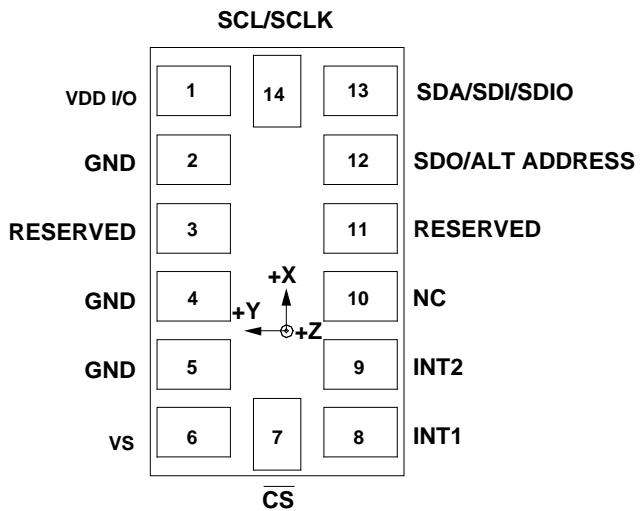
FIGURE 2. Terminal connections.
