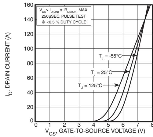
Figure 4, Transfer Characteristics
