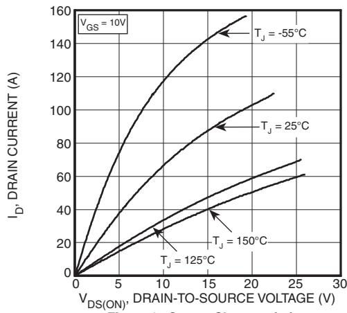
Figure 1, Output Characteristics
