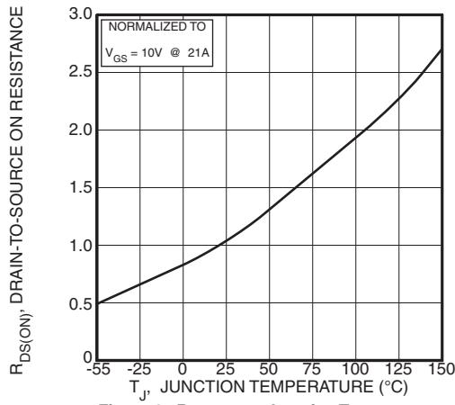
Figure 3,  $R_{DS(ON)}$  vs Junction Temperature
