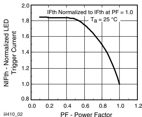
Fig. 2 - Normalized LED Trigger Current vs. Power Factor
