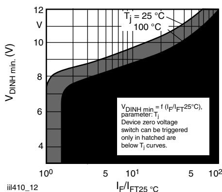
Fig. 12 - Typical Static Inhibit Voltage Limit
