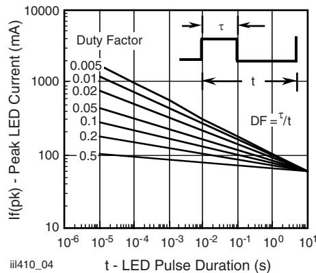
Fig. 4 - Peak LED Current vs. Duty Factor,  $\tau$
