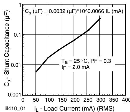
Fig. 1 - Shunt Capacitance vs. Load Current
