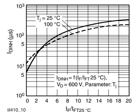
Fig. 10 - Typical Inhibit Current
