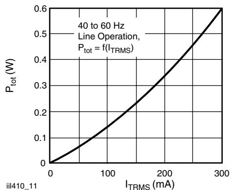
Fig. 11 - Power Dissipation 40 to 60 Hz Line Operation
