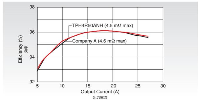
\* Test conditions: 120-W full-bridge,  $V_{IN} = 48$  VDC,  $V_{OUT} = 12$  V same MOSFET on both the primary and secondary sides (four MOSFETs in two parallel circuit branches on the primary side)
