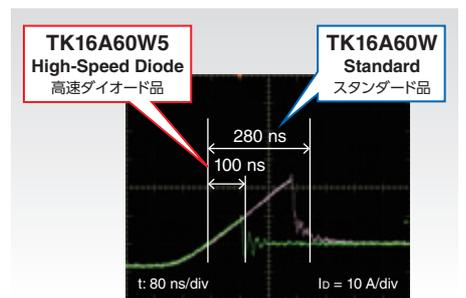
\* Test condition:  $V_{DD} = 400 \text{ V}$ ,  $I_{DR} = 7.9 \text{ A}$ ,  $T_c = 25^\circ \text{C}$
