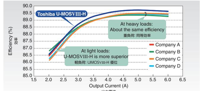
\* Test conditions: 120 W adapter, V<sub>IN</sub> = 100 VAC, V<sub>OUT</sub> = 19.5 V, critical conduction mode (CRM)
