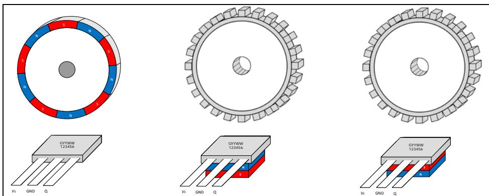
**Figure 2-1 Sensor assembly**
