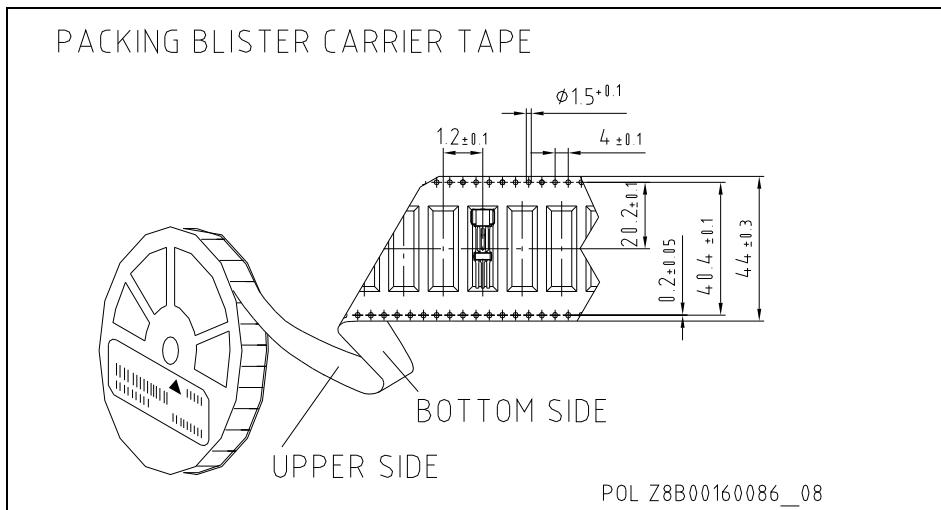
**Figure 4-8 PG-SSOM-3-11 blister tape packing information -TLE4924CB-2 E6547**
