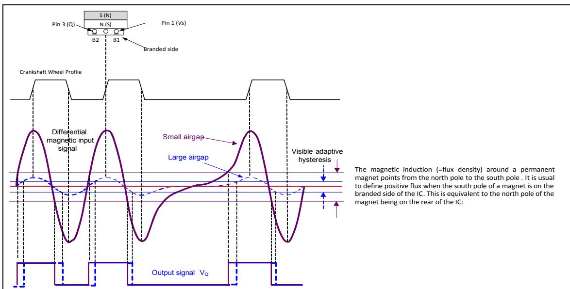
**Figure 2-2 System operation with visible adaptive hysteresis**
