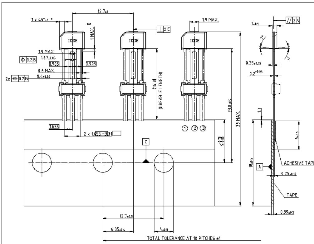
**Figure 4-5** Tape Loading Orientation in PG-SSOM-3-11 Package
