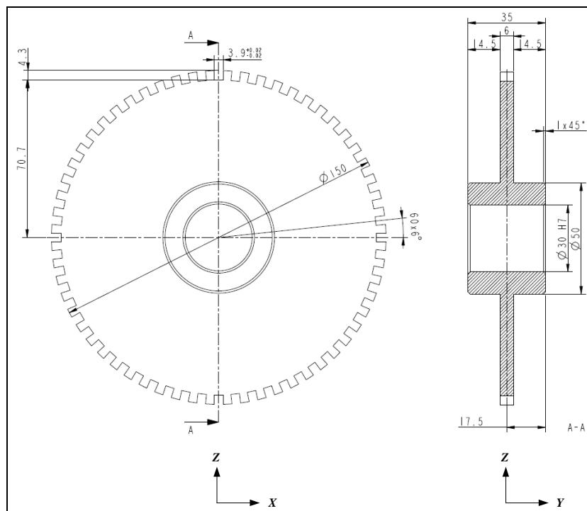
**Figure 3-1 Reference target wheel - TLE4924CB-2 E6547**
