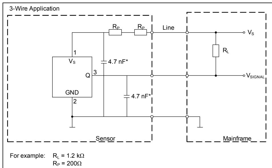
Figure 4-1 TLE4924 Application Circuits (\*capacitors included in package)
