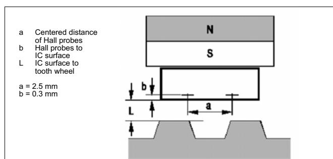
Figure 4-2 Sensor Spacing
